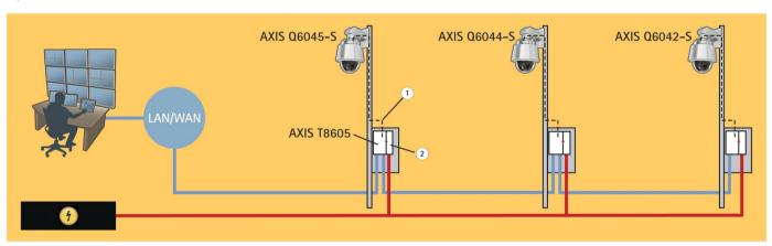
An AXIS Q60-S connects to the supplied AXIS T8605 Media Converter Switch using an IP66-rated multi-connector cable [1], which attaches to the camera with a simple click. Through the media converter switch, the multi-connector cable enables the camera to receive power (power supply [2] not included), and send and receive data to and from external alarm devices and the network. Two SFP slots and two RJ45 connectors in the media converter switch give installers the flexibility to network the
