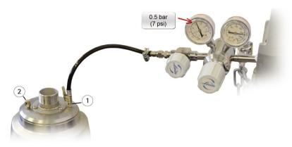
AXIS Q60-S cameras are to be filled with nitrogen gas through the inlet valve [1] and the pressure should be above 0.2 bar (3 psi) for full protection from internal condensation. The pressure relief valve [2] will open when the pressure inside the camera reaches 0.5 bar (7 psi).
